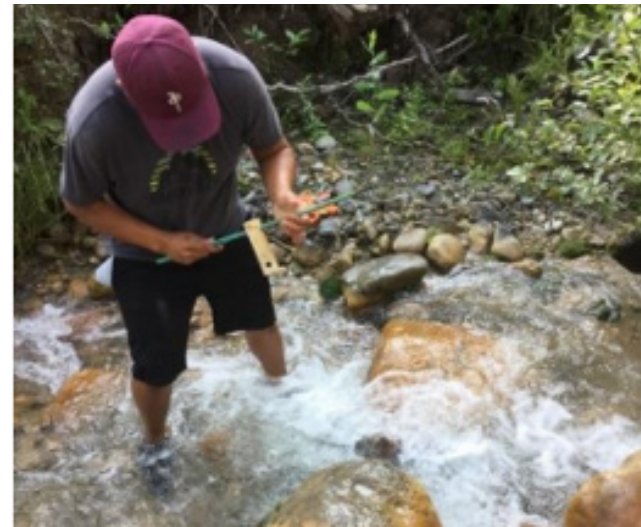
Photos courtesy of the Secwepemc Fisheries Commission. Right: Bonaparte Rivere Watershed; Left: Staff installing temperature logger.
